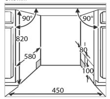
If the appliance is installed at the corner of the cabinet, there must remain enough space to open the appliance door.
