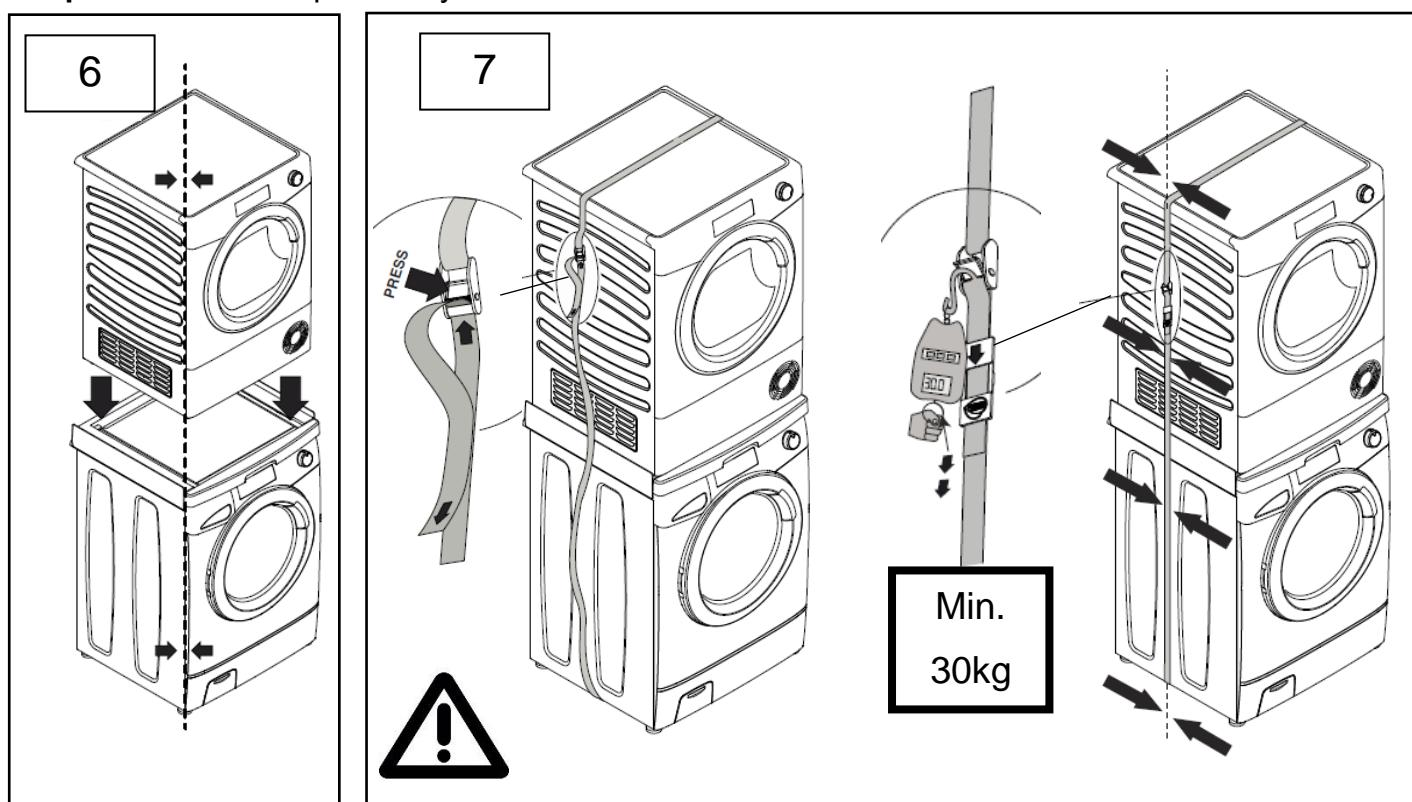
**EN:** Stack the dryer aligning the front with the washing machine (**fig.6**). Wrap the central part of the column with the belt, thread through the buckle and pull it tight (min.30kg) (**fig.7**).
