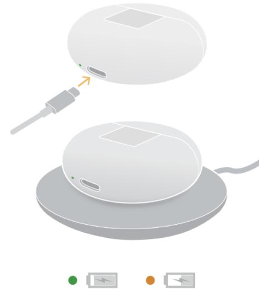
To charge the charging case, use a Type-C charger, or place it on a compatible wireless charger with the bottom facing up.
