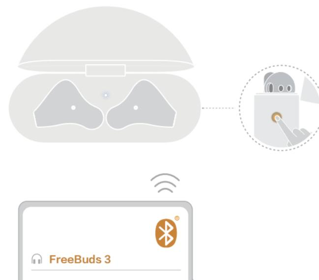
Make sure that the earbuds are in the charging case. Open the charging case, and press and hold the Function button for 2 seconds until the indicator light on the charging case starts to flash.
