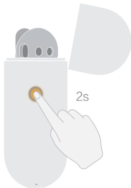
Open the charging case and press and hold the Function button for 2 seconds to power on the charging case.
